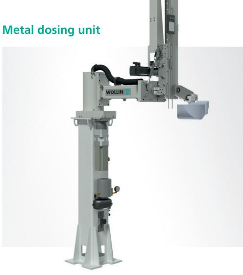
The Wollin metal dosing units **WL 1 - 4** were specially developed for automatic metal feeding of die casting machines and for gravity die casting machines up to 80 kg scoop weight. The space-saving design of the devices is achieved through an assembly stand, thereby eliminating the need for modifications to the die casting and mold spraying machine.
