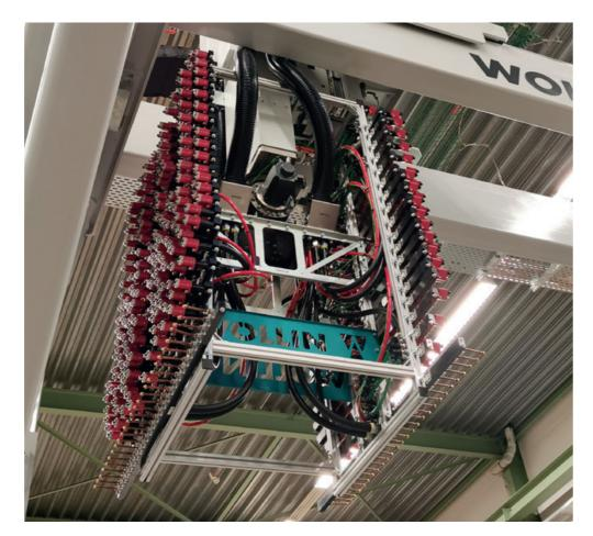
Mask spray tool for battery case
